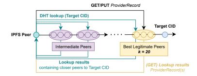
Kademlia Routing Table structure and lookup process ensure a retrieval in  $O(\log N)$  jumps (N = Network Size)
